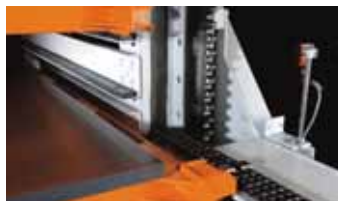
Picture 2 Shows the pallet lifter with rack and loading height control as well as the steel structure with gliders
