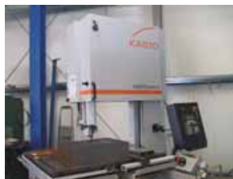
Picture 4 Shows the work range of the KASTOvertical. A material block is positioned on the movable support table ready to be cut
