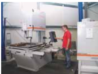
Picture 3 Shows the KASTOvertical with moving support table: Programming of orders is done easily and ergonomically by the KASTO-CompactControl
