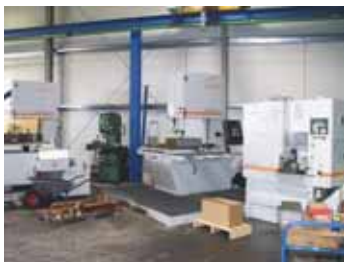
Picture 1 Shows the three Production Bandsaws at Marks: from left KASTObloc U 5, KASTOvertical, KASTOssb 260
