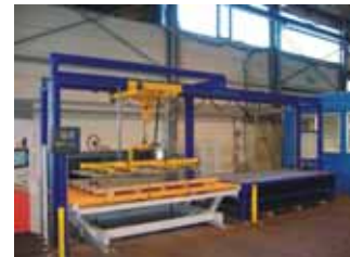
Picture 3 Shows the commissioning location for sheet metal with a lateral cart and a sheet restacking system
