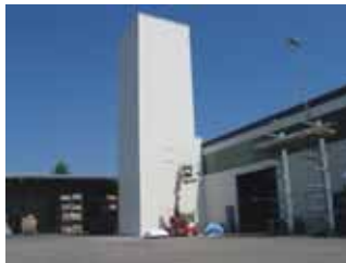
Picture 1 Shows the UNITOWER Storage System for sheet metal docked to the outside building wall at Damstahl
