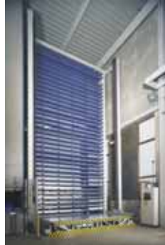
Picture 2 Shows a one-sided Sheet Metal Storage and Retrieval System UNITOWER B for maxi sizes (4 x 2 m) with a usable load of 3 tons per pallet
