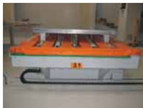
Picture 4 Shows the station cart of a Sheet Metal Storage and Retrieval System UNITOWER B at a steel distributor taking out the stored material
