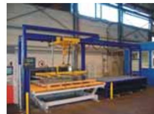
Picture 6 Shows the commissioning area of sheet metal with a lateral cart and a sheet metal restacking system for commissioning at a steel distributor
