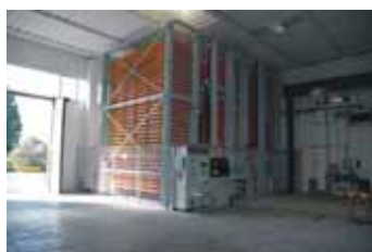
Picture 7 Shows a double-double tower with station cart and EasyControl at a steel distributor
