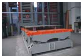
Picture 8 Shows a cart moving longitudinally out of a double-double tower with scale and raised sheet pack
