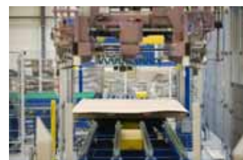
Picture 9 Shows a fully automatic sheet metal commissioning system at a large steel distributor in Denmark
