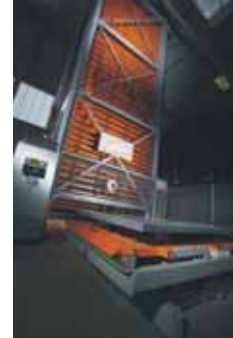
Picture 3 Shows a Sheet Metal Storage and Retrieval System UNITOWER B as double tower with lateral cart and lift unit at a steel distributor
